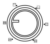
**Temperature Control Knob:** This knob helps to set the desired temperature for the particular recipe. Temperature range is from Min. to 100°C to 230°C.
